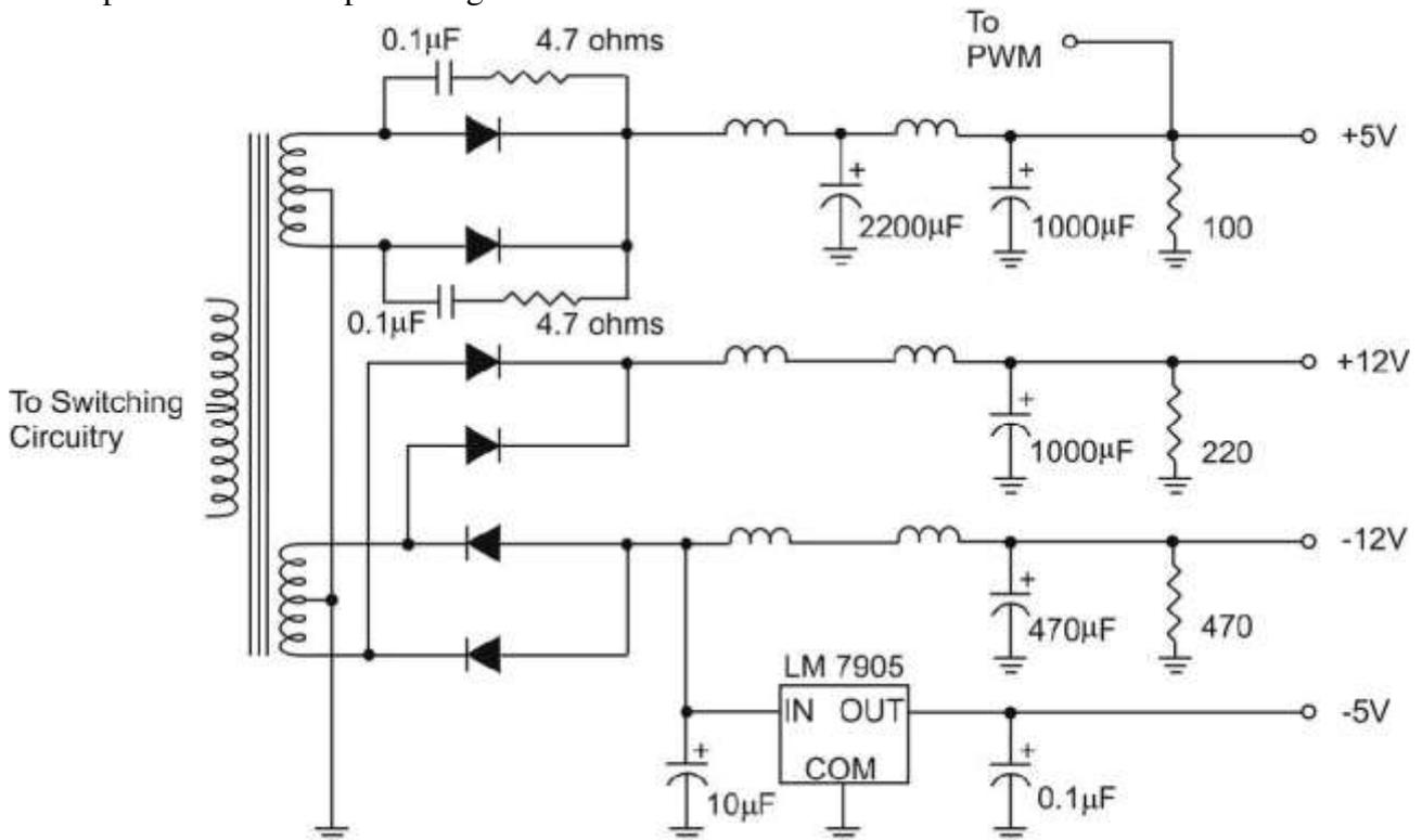
Key to the success of this design is a multiple secondary power transformer. There is a 5-volt winding and a 12-volt winding. In high-power supplies (250 watts and larger), there are usually two five-volt windings that are paralleled for higher output current—yet treated as a single winding.
