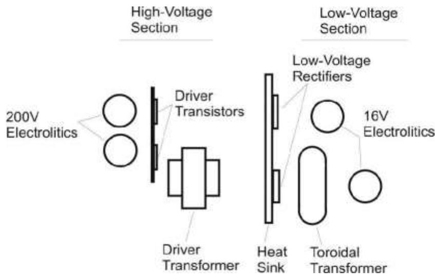
An ohmmeter is a good way to probe suspected areas for shorted devices. It's virtually impossible to tell the difference between a shorted diode and a shorted capacitor without removing one or the other. Since the rectifier is the most likely culprit and the easier to remove (the electrolytics are glued in place), you can start there.
